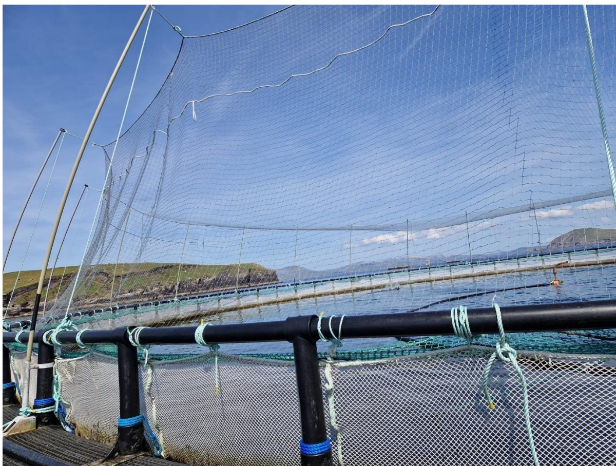
Figure 22. Seal ingress protection netting exterior view
